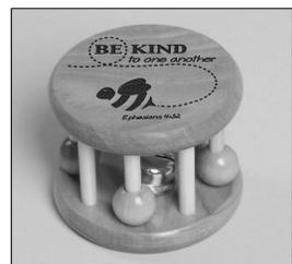
**PROBLEM:** The wooden dowels can be installed at an angle, allowing the metal rattle inside to become exposed. This poses a serious choking hazard to young children.
